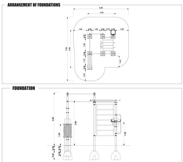
Each vertical column poured with semi-dry concrete C20/25 for 80 cm below ground level. Volume of one footing min. 0,125m<sup>3</sup>. Fundations are placed 30 cm below ground level, what prevent accidential or purposeful discovery.
