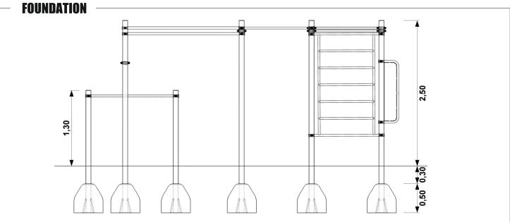
Each vertical column poured with semi-dry concrete C20/25 for 80 cm below ground level. Volume of one footing min. 0,125m<sup>3</sup>. Fundations are placed 30 cm below ground level, what prevent accidential or purposeful discovery.
