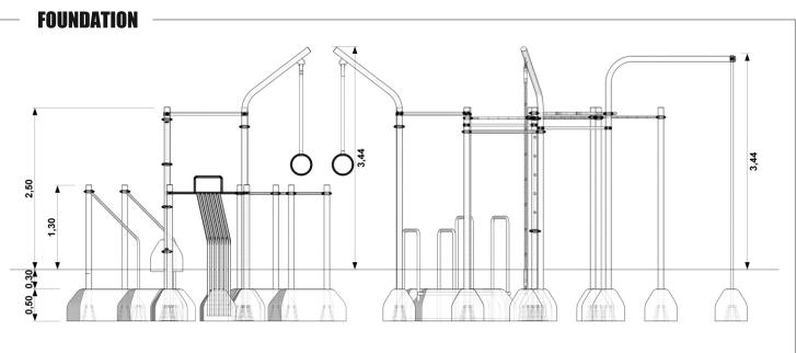
Each vertical column poured with semi-dry concrete C20/25 for 80 cm below ground level. Volume of one footing min. 0,125m<sup>3</sup>. Fundations are placed 30 cm below ground level, what prevent accidential or purposeful discovery.
